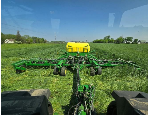
Drilling soybeans no-till into standing cover crop. Nicollet County SWCD
