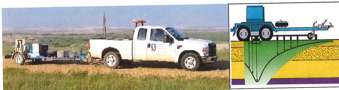
Figure 1 Dynatest 8002 FWD Test System
